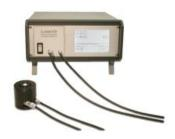
The photocell, which is supplied mounted on the rotating arm, is connected to the luxmeter by a shielded cable of a maximum length of 70 m: should it be necessary to increase this distance, a suitable signal amplifier will have to be taken into consideration.
