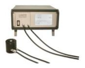
The photocell is thermostatized at 35°C and is supplied along with a support to be fixed to the floor or ceiling.
