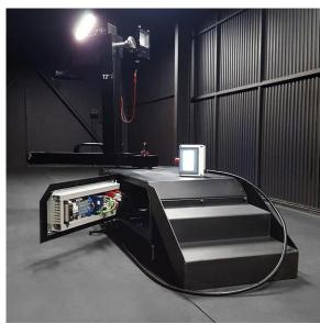
The angular resolution of the encoders is equal to 4/100° (13 bit) and the angular positions are shown on screen during measurement along with indication of the state of
